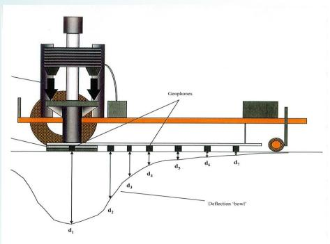
Falling Weight Deflectometer Schematic
